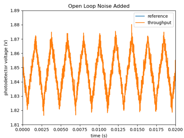
(a) Open-loop control demonstrating the added triangle wave disturbance.
