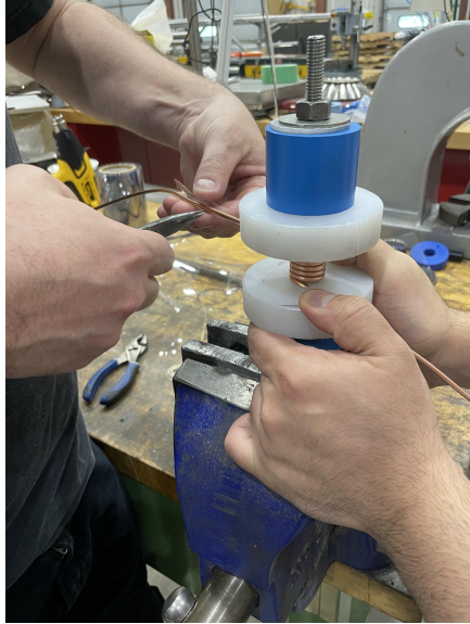
(a) The jig used to wind the coils
