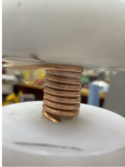
(b) The plastic insulation between winds. Notice the 'canoe' on the inter-layer wind.
